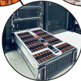
7.5 PB disk tier (OST) 8 x Western Digital Data60 22TB SED
